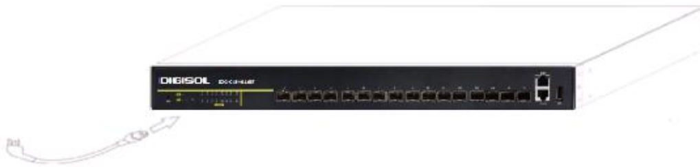
Fig 2- 4 Attaching power cable to DG-CS4616F
