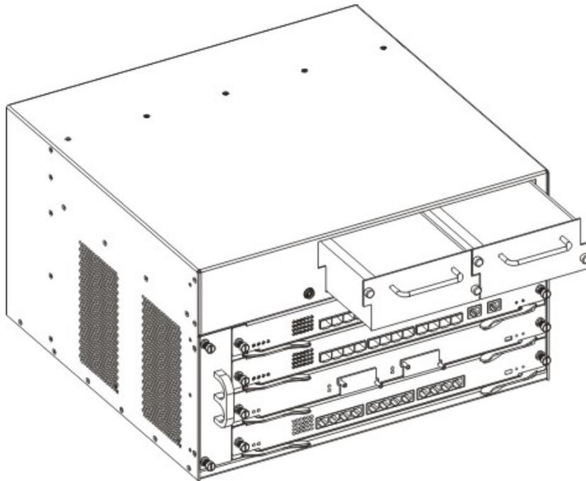
Fig 2-9 The installation and removal of DG-CS7004 power supply modules
