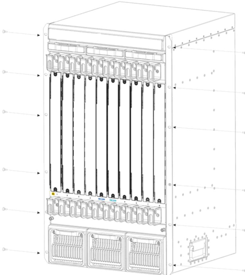
Fig 2-2 Installing DG-CS7010 Switch Hangers
