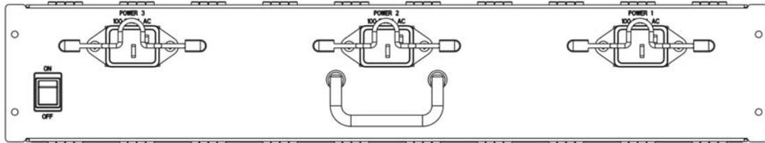
Fig 1-29 DG-CS7010 AC Power Distribution Box
