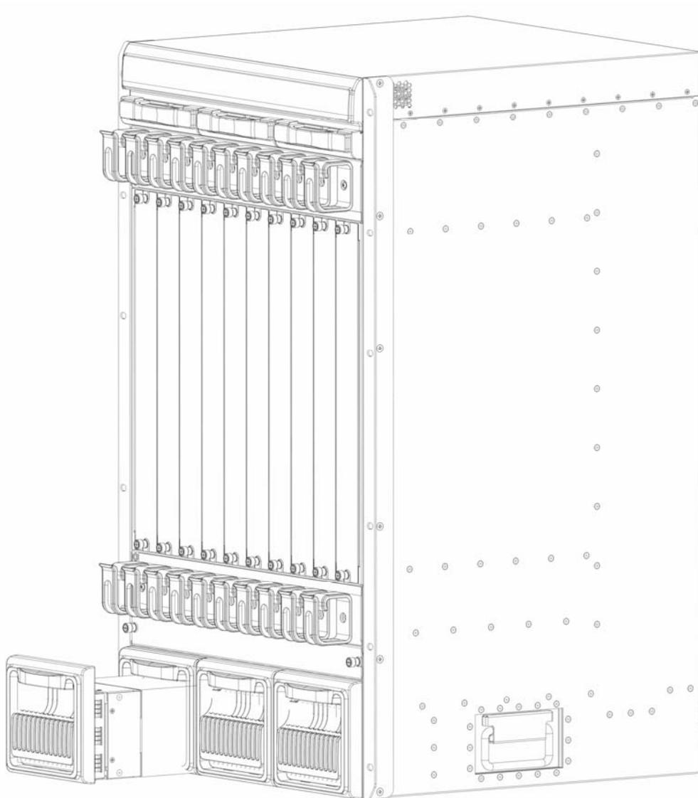
FIG 2-10 The installation and removal of DG-CS7010 power supply modules
