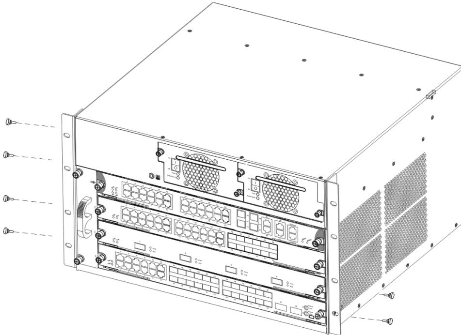
Fig 2-1 Installing DG-CS7004 Switch Hangers
