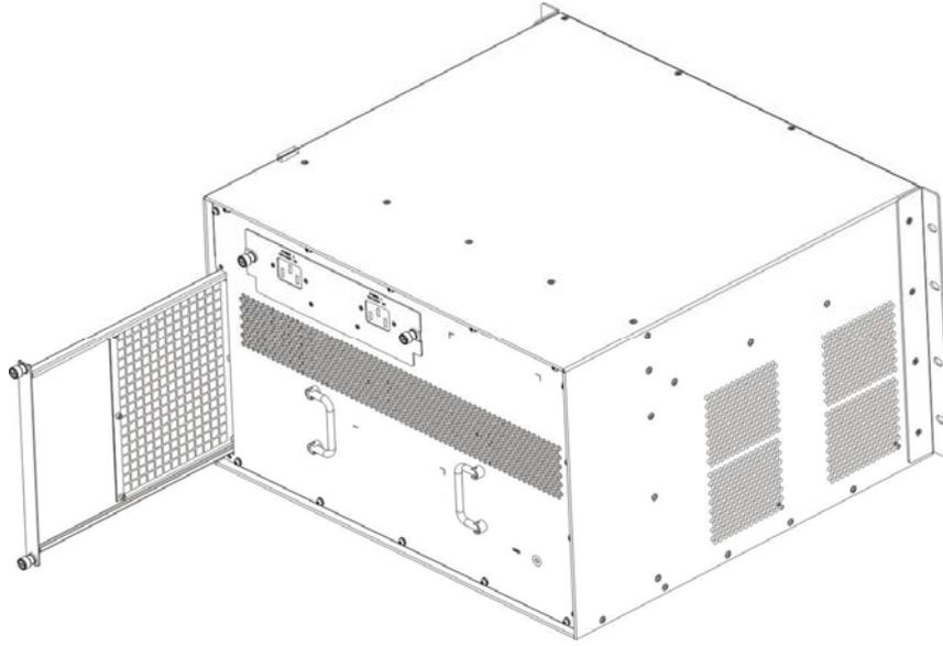
Fig2-5 Installation and removal of the DG-CS7004 dust gauze
