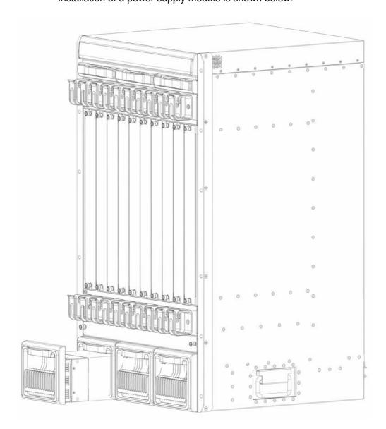
FIG 2-10 The installation and removal of DG-CS7010 power supply modules
