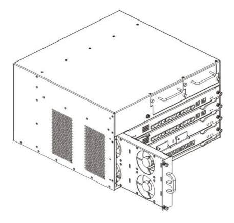
Fig2-7 The installation and removal of DG-CS7004 fan tray
