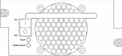
Fig 1-25 DG-SA-RPS-7004AC Front Panel View
