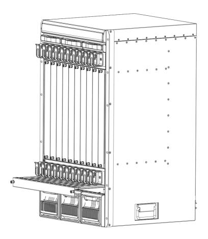
Fig2-6 Installation and removal of the DG-CS7010 dust gauze
