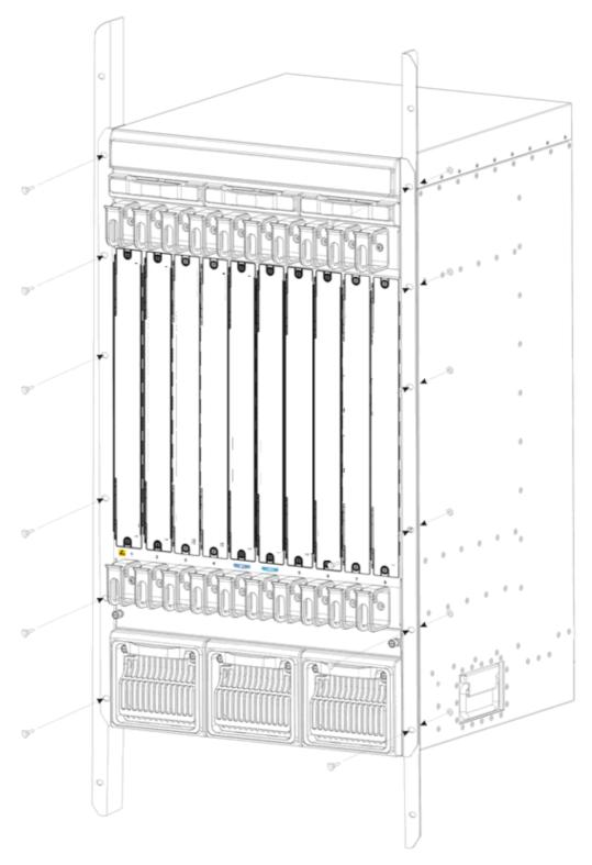
Fig2-4 Rack-mounting DG-CS7010
