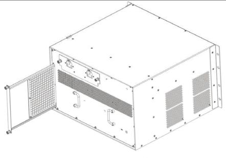
Fig2-5 Installation and removal of the DG-CS7004 dust gauze
