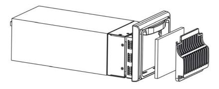
FIG 2-11 The installation and removal of Power module dust gauze
