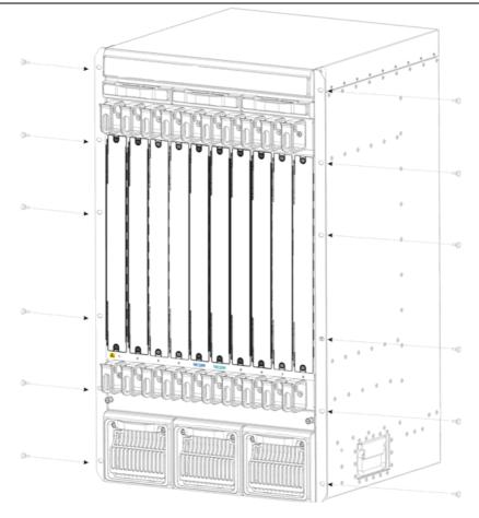
Fig 2-2 Installing DG-CS7010 Switch Hangers
