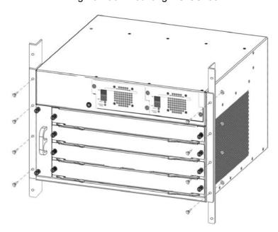
Fig2-3 Rack-mounting DG-CS7004
