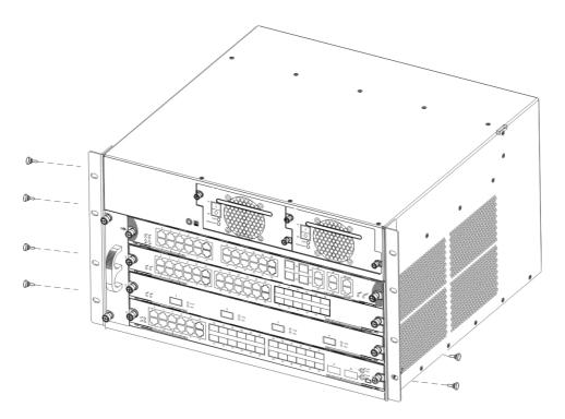
Fig 2-1 Installing DG-CS7004 Switch Hangers
