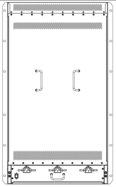
FIG 1-37 DG-CS7010 Rear Panel View
