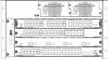
Fig 1-4 DG-CS7004 Front Panel View
