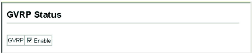
Figure 3-120 Globally Enabling GVRP
