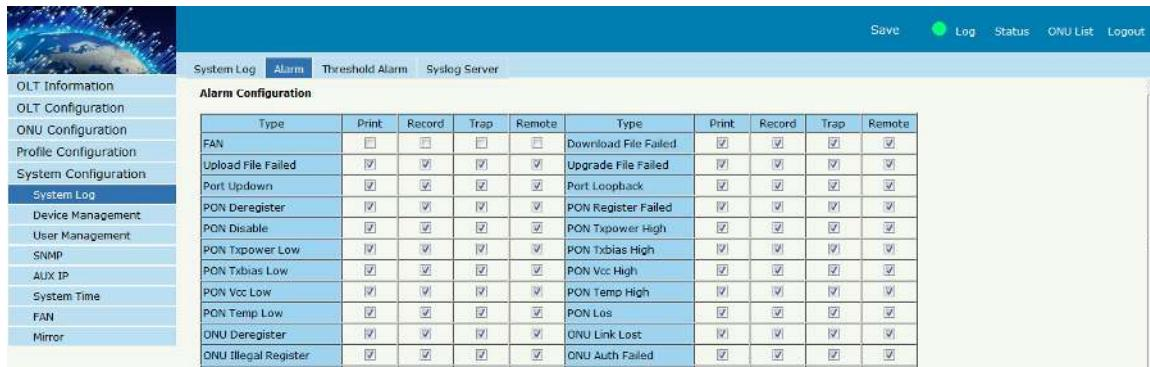
The screenshot shows the 'Alarm' tab selected in the navigation bar. The main area displays an 'Alarm Configuration' table with columns for Type, Print, Record, Trap, and Remote. The table lists various alarm types such as FAN, Upload File Failed, Port Updown, etc., each with its corresponding checkboxes for the four actions. The interface includes a sidebar with various management links and a top bar with save, log, status, and other navigation buttons.
