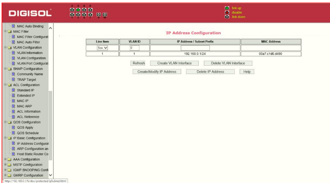
Figure 38 VLAN interface configuration page
