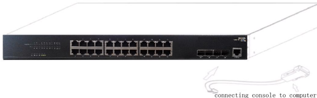
Fig 2-3 Connecting Console to switch
