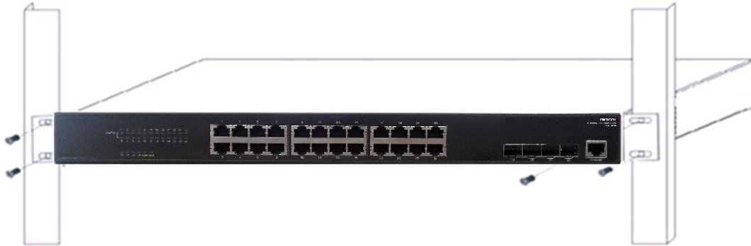
Fig 2-2 Fasten the Switch to the Rack
