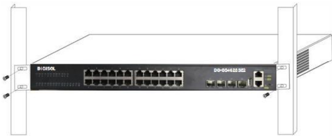
Fig 2- 1 Install sketch map on the rack
