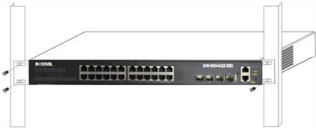
Fig 2- 1 Install sketch map on the rack
