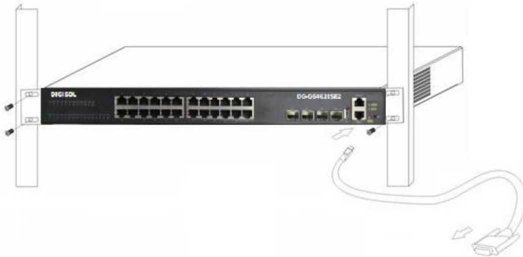
Fig 2-2 Connecting Console to switch
