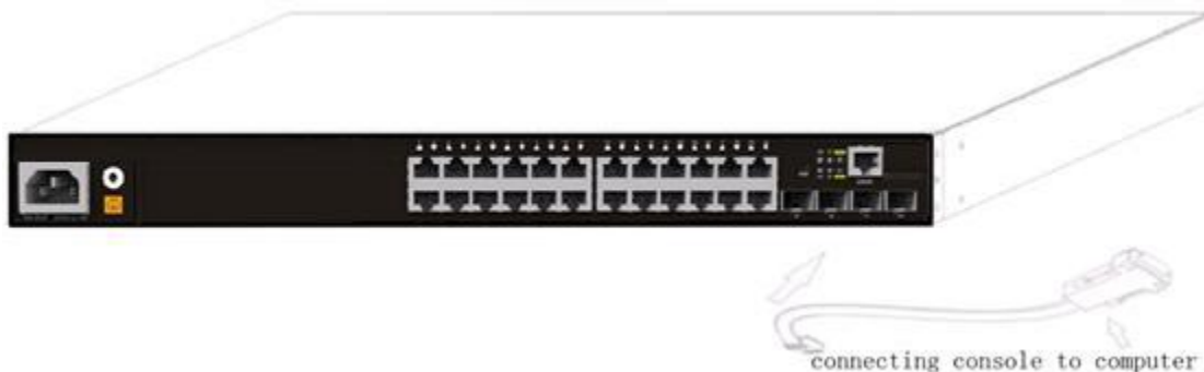
Fig 2-3 Connecting Console to switch
