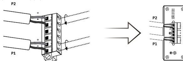
Note: please connect the positive “+” and negative “-” pole correctly according to the panel symbols under terminal block, and put in the right power voltage. 24VDC is recommended.
