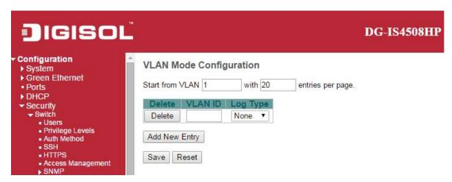
Specify ARP Inspection is enabled on which VLANs. First, you have to enable the port setting on Port mode configuration web page. Only when both Global Mode and Port Mode on a given port are enabled, ARP Inspection is enabled on this given port. Second, you can specify which VLAN will be inspected on VLAN mode configuration web page. The log type also can be configured on per VLAN setting.
