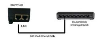
Step3: Connect CAT5/5e/6 cable from PoE enabled device (e.g. PoE IP camera or a PoE Access point) to the "PoE" port on DG-PE1148D.
