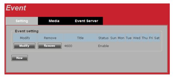
When there's an event, you can use this setup page to define what IP camera should do, like send an Email or trigger digital output to activate external alarm.
