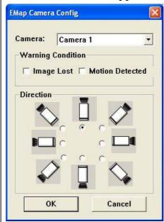
Select the camera you wish to add from 'Camera' dropdown list, and check the box 'Image Lost' and / or 'Motion Detected', then select the direction of camera icon, this will help you to remember the
