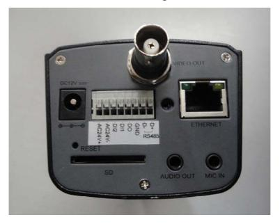
This Ethernet port supports IEEE 802.3af PoE standard. It gets power when it is connected to PoE switch.
