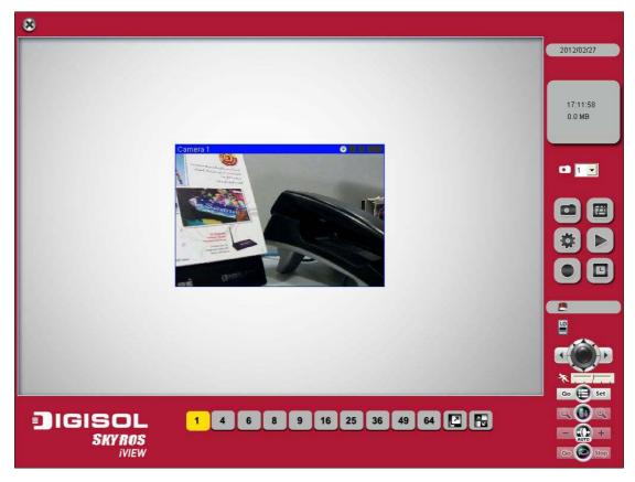
(This example picture shows a camera view with only 1 IP camera configured) To select an IP camera, click its video and it will be highlighted; some IP cameras support additional control, and a control panel will appear at the bottom right area of SKYROS iView.
