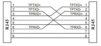
Choose the connection which best fits the connection between switch and other Ethernet terminal. 10/100Base-TX port and other Ethernet terminal connection is shown as follows:
