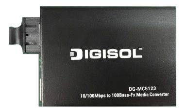
**DIGISOL** Media Converter can interconvert electrical signals of 10Base-T and 100Base– TX twisted pairs with optical signals of 100Base-FX. It extends the network transmission distance from 100m via copper cables to 20km via fiber optical cable. It enables the data to transmit in two different mediums of electrical and optical networks either by the technology of data link L2 store-and-forward, or by the one of PHY L1 cut-through. It supports transmission in single-mode dual fiber.
