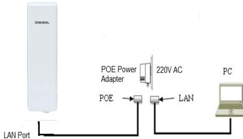
**Fig. 2 Diagram of PoE Power and AP configuration**
