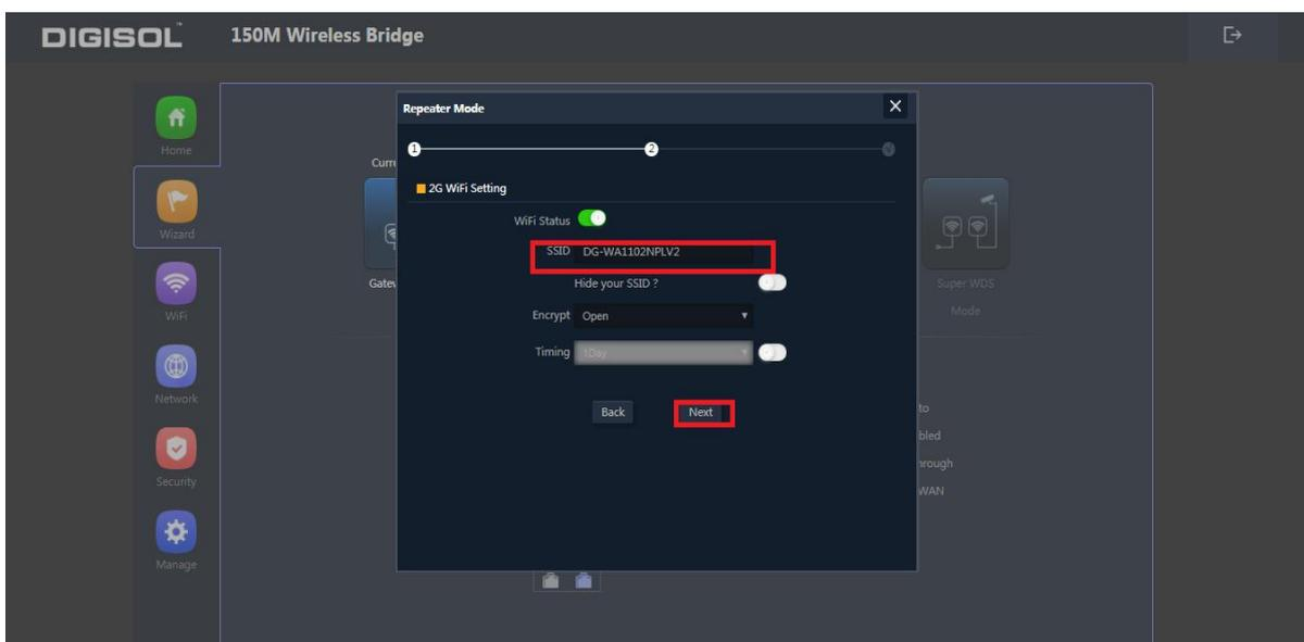
**Fig. 21 Wireless Setting in Repeater Mode**
