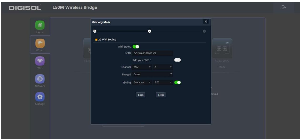
Fig. 17 Wireless Setting in Gateway Mode
