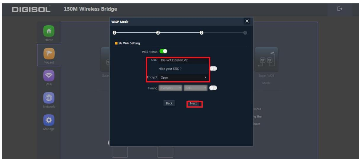
Fig. 26 Wireless Setting in WISP Mode
