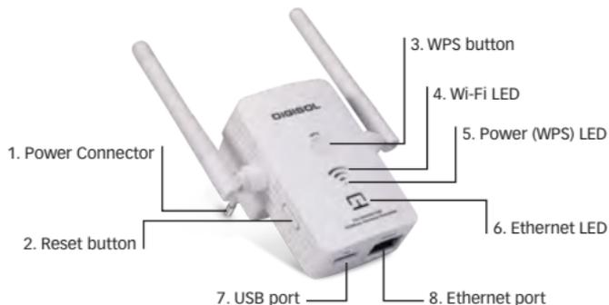
This wireless range extender includes Wireless AP, Wireless repeater, and USB Port for charging other devices.
