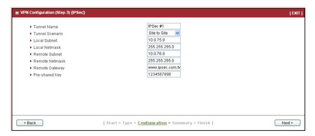
"Dynamic VPN" is for remote users to connect to the device securely. For other options, please go to Advanced Network >> VPN to setup. Input the required network information and pre-shared key for VPN connection.
