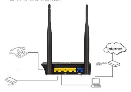
4. Please check all LEDs on the front panel. Power LED 'PWR' should be steadily ON, WAN and LAN LEDs should be ON. Check if the computer/network device connected to the respective port of the router is powered ON and correctly connected. If power LED 'PWR' is not ON, or any LED you expected is not ON, please recheck the cabling.
