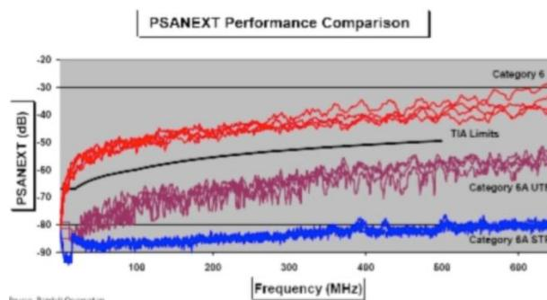
A key determinant of the type of CAT 6A to be used is a study of EMI intensity in the industrial environment where they are being installed. In industries, EMI can be caused by a host of factors including nearby air conditioners, electrical motors and even office equipment like desktops, printers and fluorescent lights. EMI generates ANEXT (Alien Near End CrossTalk) in circuits, degrading data quality, slowing down transmission and spiking error rates.
