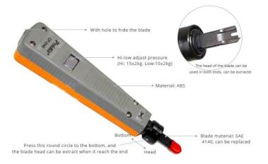
It has always worked perfectly for 110-type patch panel and keystone jack installations so far. It involves using this hand tool to "impact punch" the ethernet cable wires into the IDC (Insulation Displacement Connectors) on the punch down blocks, patch panels, and keystone jacks.
