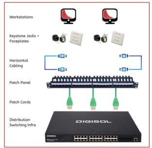
Aesthetically enclosed within your office furniture and civil infrastructure, keystone jacks combined with faceplates connect the workstations to patch panels using horizontal ethernet cabling.
