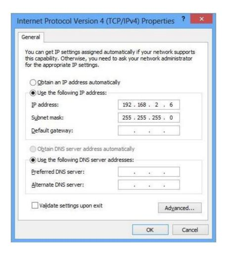
Also, make sure that your network address does not conflict with the DG-HR3400. If your existing wireless network has 192.168.2.1 IP assigned in your network it is recommended to change the IP of DG-HR3400 from 192.168.2.1 to 192.168.2.x (x stands for any digit between 2-254 which is not used in your network).
