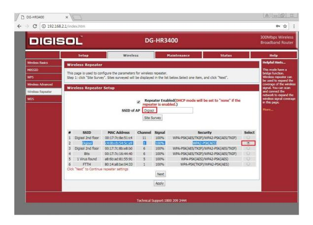
Now as shown below in the next screen enter the security key. This key should match with your existing wireless network TEST which we have used in example. Click Apply to continue with the setup.
