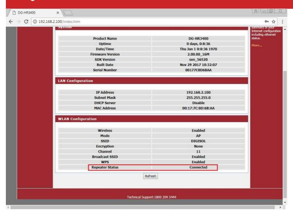
After the device has completed the rebooting process check the Repeater status as shown in below screen shot . Click on Status. Status should be Connected if it is successfully connected to your network as shown in the below screen.
