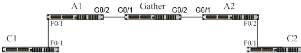
A1/A2/Gather belongs to a core network. C1/C2 stands for two switches locating in two branches of a customer. The customer wants the two networks to be managed as an independent network, that is, the core network is just like a transparent transmission channel for this customer. To realize STP transparent transmission, the customer needs to make the following settings on each switch:
