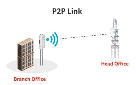
Use a DG-WA5ACL20 on each side of a Point-to-Point (PtP) link.
