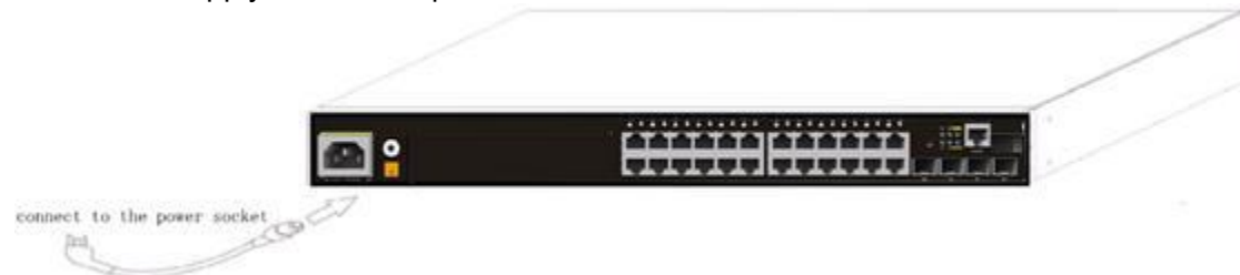
Fig 2-4 Connecting power to switch
