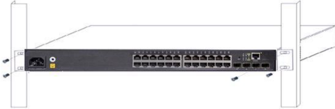
Fig 2-2 Fasten the Switch to the Rack
